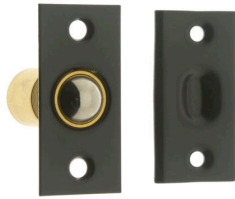
#12010 Narrow Square Roller Ball Catch Face: 1" x 2-1/8" Strike: 1-1/16" x 2-1/8" Tube Diameter: 3/4" Tube Length: 1 1/2"
