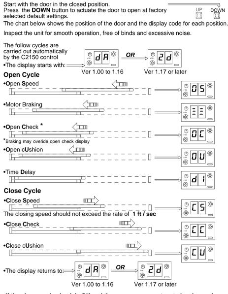
•If the above cycle check is OK and there are no parameters to be changed or an autolock to setup, this concludes the C2150 initialization.
