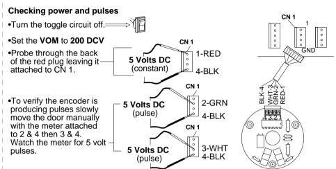
If the above voltages check out and the display does not rotate as shown in section 12 then contact the technical services group.
