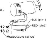
NOTE: A low reading is critical and will cause damage to the control.
