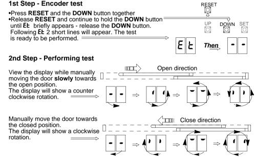
Each segment of 4 for a total of 8 segments should appear. No segment should be skipped. If anything occurs other than the description shown above the C2150 will get improper information and the door will not function properly.
