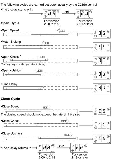
•If the above cycle check is OK and there are no parameters to be changed or an autolock to setup, this concludes the C2150 initialization.
