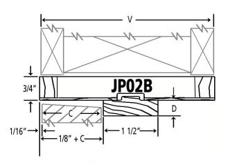
MINIMUM WALL WIDTH 4-5/8" NON-RATED, 20 MIN, 45 MIN, 60 MIN, 90 MIN 1/2" stop height standard for non-rated 5/8" stop height required for rated
