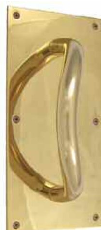
OLYMPUS - Plate-12"L x 6"W Pull-8-1-1/4"CTC 1"D Bar pull, 1/8" bronze sheet plate.
