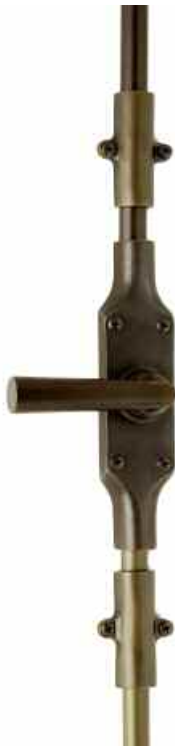
MIDDLETON - 1-9/16" x 6-13/16" x up to 120" door Specify hand. Cast bronze cremone bolt.
