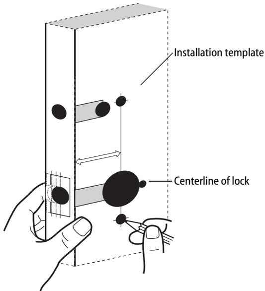
Figure 1 Positioning the template
