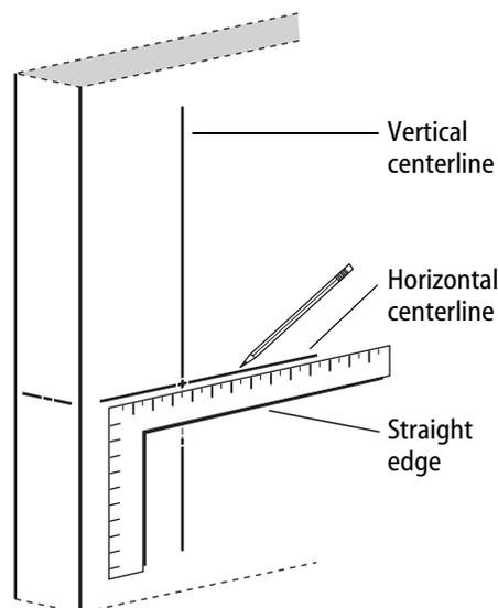
Figure 1 Marking centerlines on outside door face
