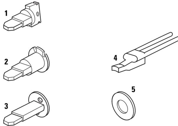
**Figure 4.3** Lever components for use with non-interchangeable cores
