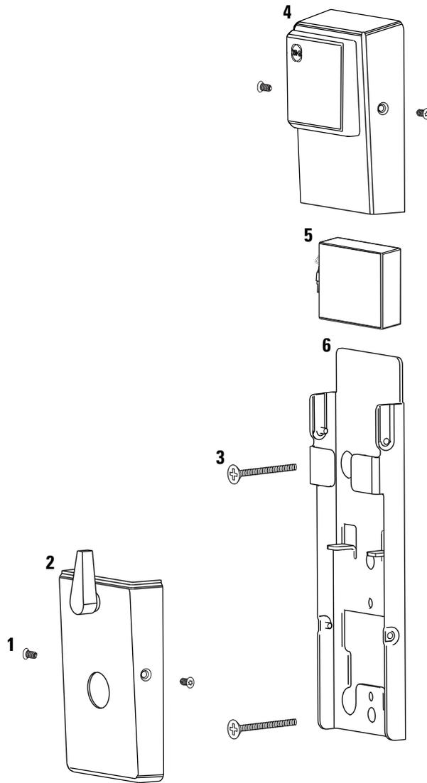
**Figure 2.1** Inside escutcheon components (mortise TV function shown)
