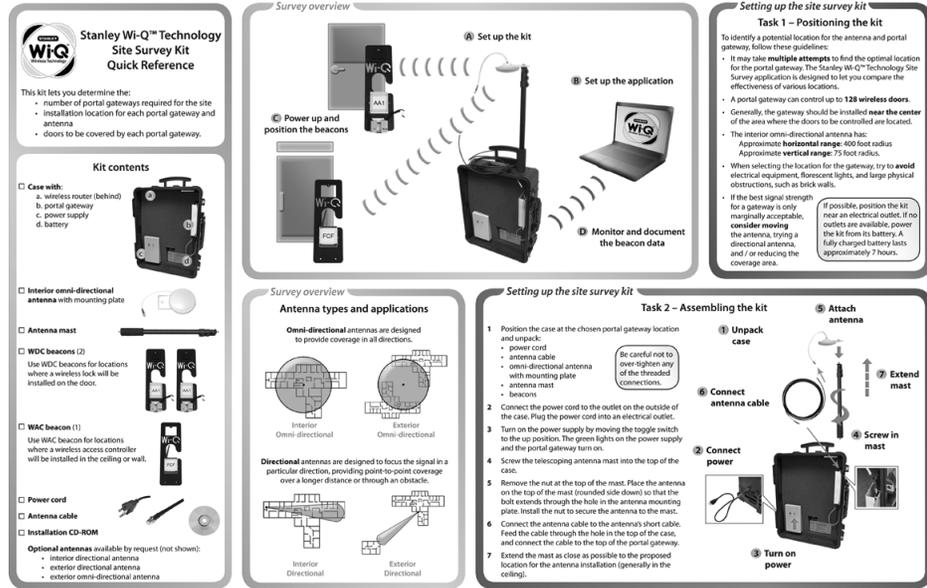
Figure 7.7 Site survey kit and beacons components
