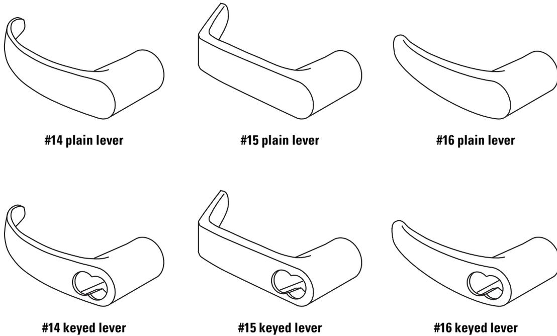
**Figure 4.1** Cylindrical levers
