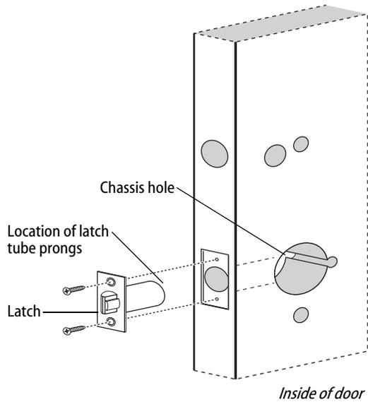
Figure 3 Installing the latch in the door
