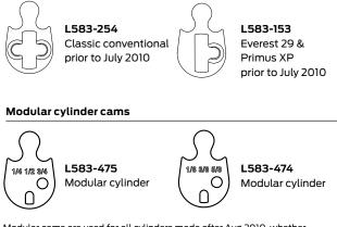
Modular cams are used for all cylinders made after Aug 2010, whether Classic, Everest 29 or Primus. L583-474 is used on cylinders 1 1/8", 1 3/8" and 1 5/8". L583-475 is used on cylinders 1 1/4", 1 1/2" & 1 3/4".
