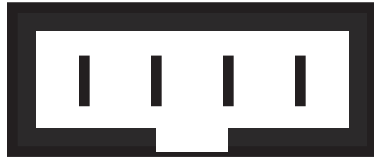
Figure 4-2: J4 - RS-232 Jack Pinout
