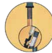
When check pin is lifted, cylinder is free to rotate
