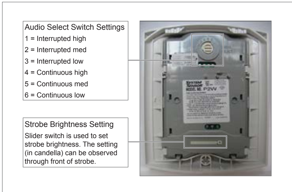
Figure 1, Location of Setting Switches (back of horn strobe)
