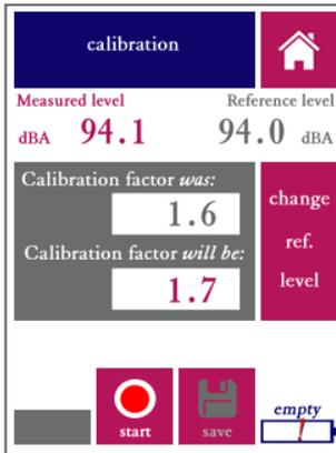
*Calibration module showing calibration results.*
