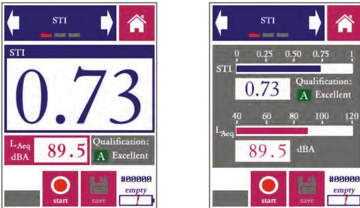
*STI measurement screen of the Quick STIPA module, in digit mode (left) and bar mode (right)*
