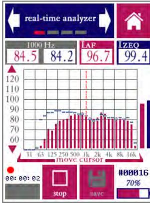
*RTA main measurement screen (1/3 octave band mode)*
