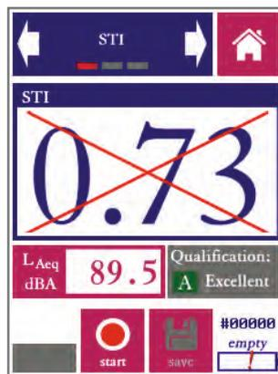
*A crossed-out STI value means that the measurement is not (yet) sufficiently reliable*
