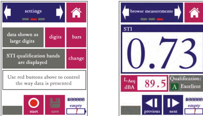
“Settings” screen and “browse measurements” screen. The latter screen is nearly identical to the STI measurement screen, but with previous/back buttons instead of start/stop and save buttons.
