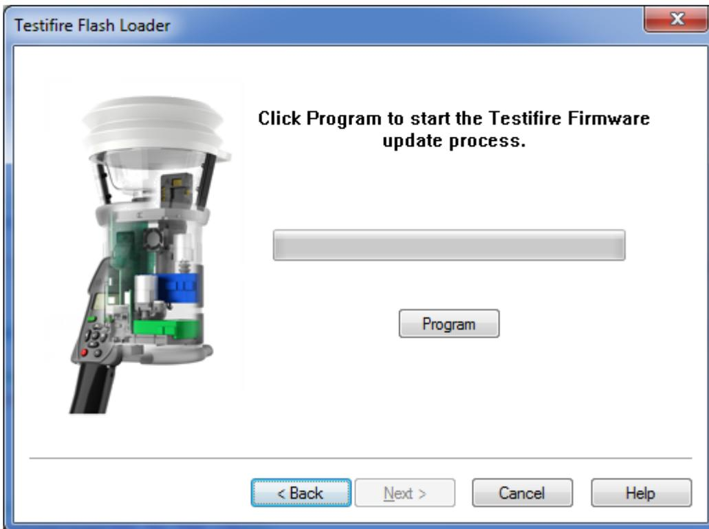
**Do not interrupt programming or disconnect the USB cable.**
