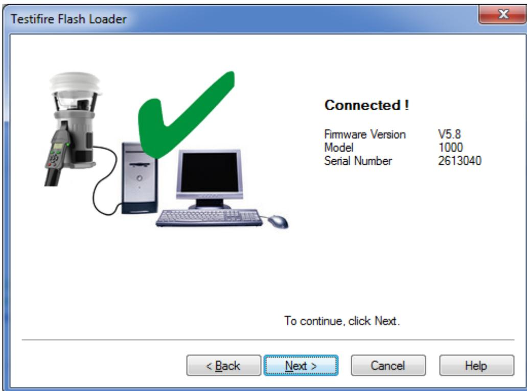
If the Testfire is not detected instantly, the scanning process will continue until either the Testfire is detected or the user clicks on Back or Cancel buttons.
