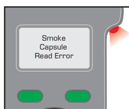
Capsule damaged or not seated correctly.
