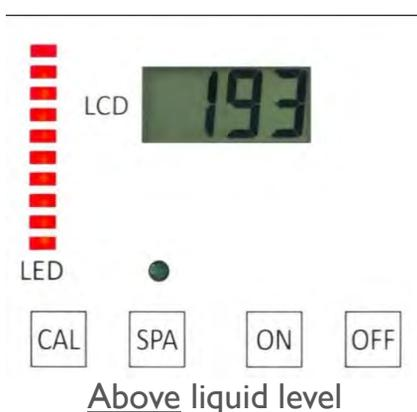
Step 4: Move sensor 5cm down, observing the bar graph
