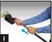
1 Insert a charged battery baton into the tool and pole.
