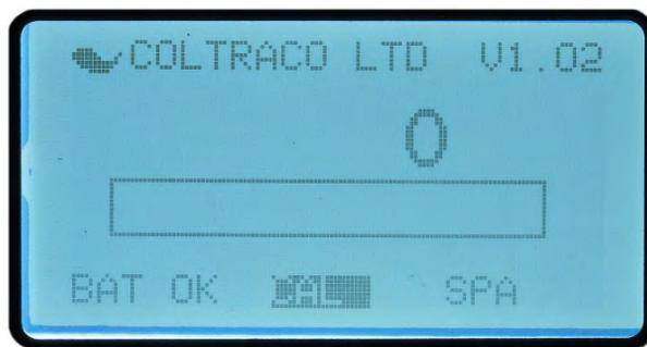
Then disengage CAL by pressing the CAL button again and turn the unit off. This completes the Function Test.
