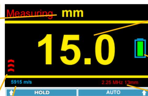
**Digital Display:** Numerical readings allow users to determine the thickness of the material
