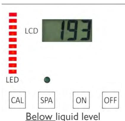
Step 4: Move sensor 5cm up, observing the bar graph
