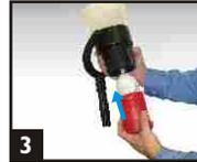
3 Replace retainer cup and screw upwards. Adjust until aerosol activates and unscrew slightly.
