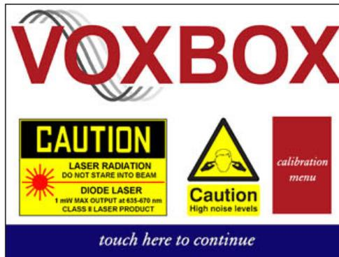
Press on the blue bar at the bottom of the screen to skip directly into the main menu. Press the button “calibration menu” if you need to adjust the level calibration of the VOXBOX or to change any of the hardware settings. See section 3.3 for a description of these settings.
