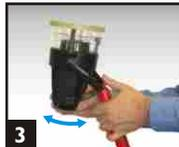
3 Position the latch and place over detector.
