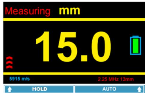
When the battery is indicated to be low on power, the battery must be replaced before it is used further, or the unit may provide anomalous results.
