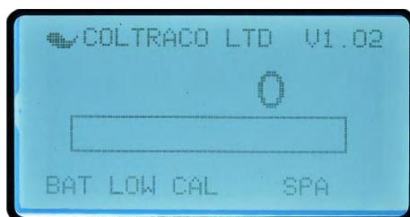
When the battery low indicator is displayed, the battery must be replaced before it is used further, or the unit may provide anomalous results. To replace the battery follow the instructions overleaf.
