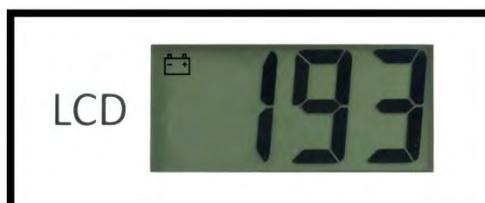
When the battery low icon is displayed, the battery must be replaced before the unit is used further.
