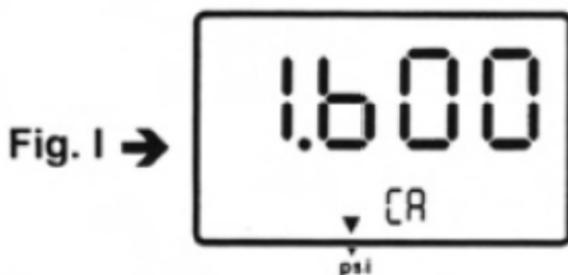
4. The meter has defaulted to 1.6 psi calibration point, the adjustable pressure range is from 1.5 to 1.7 psi. If calibration pressure source is not 1.6 psi, increase by pressing **DIF** key, or decrease by pressing **Ⓢ** key to set calibration point as required.
