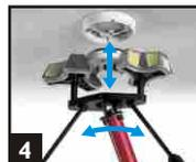
4 Grip detector, twist and pull down to remove.
