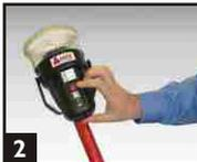
2 Press the red switch to turn on. LED illuminates green. Flash at slow rate indicates normal STANDBY mode.
