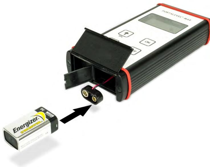
Step 6: Close battery cover, ensuring that the wires are not trapped.
