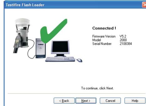
If the Testifire is not detected instantly, the scanning process will continue until either the Testifire is detected or the user clicks on Back or Cancel buttons.
