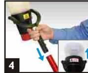
4 Insert the Solo 330 into Solo pole. Place Solo 330 over the detector and press upwards to activate the aerosol (1 second burst).
