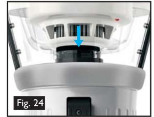
**TIP:** To prevent Testifire going straight into a test mode, both the inner and outer clear cups should be cleaned regularly with a damp non-abrasive cloth to remove any deposits or finger marks.
