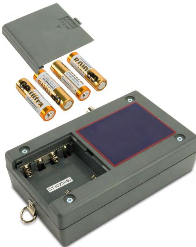
Step 3: Place battery hatch back into housing and gently slide into place.
