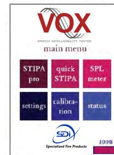
From the main menu, you can launch apps for the instrument's different measuring modes, as well as apps that let you calibrate the device and control its settings. All modules make use of an intuitive graphical user interface utilizing the VOX-01's color touch screen. This gives all modules a consistent look and feel, which will allow you to familiarize yourself with the device with ease.
