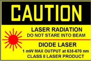
The VOXBOX features a class II laser pointer to assist in placement of microphones. Never look directly into the laser, and make sure that others cannot accidentally look directly into the laser either. Do not use around children or animals. Do not disassemble or remove the laser from its enclosure.
