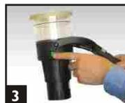
3 Connect to power and press ON switch. Place over detector.
