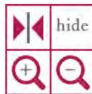
These controls are used to zoom in or zoom out along the frequency axis, and to center the display around the current cursor position. By pressing “hide” the zoom controls are collapsed again. The zoom controls are used together with the cursor to focus on any region of interest in the spectrum.. The cursor, shown as a vertical red line, can be moved by tapping the arrows below the frequency axis or by tapping directly on the graph.
