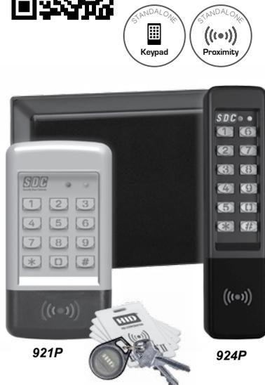
The 921P and the 924P EntryCheck™ stand-alone digital keypad with Prox Reader and Controller (2-piece configuration) are designed to control access of a single entry point with up to 500 users. Each user is assigned a personal identification number (PIN). Keypad entry of a valid one to six digit code activates one or both of the output relays which releases an electric door lock. Heavy Cast Vandal Resistant Housing. Heavy Cast Metal Blue Backlit Keys.
