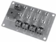
**FB4DC** AC to 4 DC Fused Output Module. One (1) AC input, 12 or 24VAC 4.2 Amp max. Four (4) Fused DC outputs (4) Fuses, 2 Amps. Combined load of all outputs 4.2 Amps max. **60.00**
