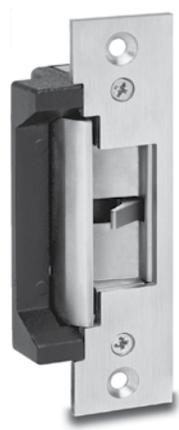
The SDC 25 Series electric strike is designed for use with locksets having 5/8" (15mm) throw latchbolt. The compact low profile design with an internally mounted solenoid and factory supplied mounting tabs enable quick and easy installation where jamb space is limited.
