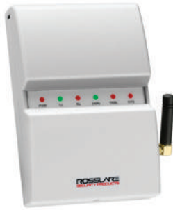
Wireless Access Control Door Interface Near Unit
