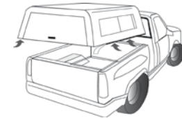
Sponge Vinyl Camper Tape installed as seal between camper and truck bed
