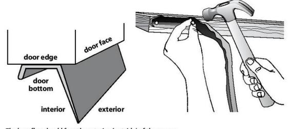
The long flap should face the exterior (outside) of the garage.
