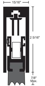
Designed for use on sliding or pocket doors. A series of actuating bars keep the seal parallel to the sill or threshold until the door is in the closed position.
