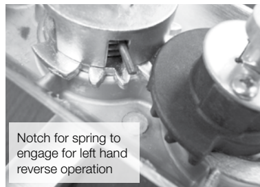
Spring orientation for right hand reverse operation
