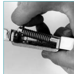
3. Grasping adjustment pin, compress spring and place adjustment bushing assembly over round pin.
