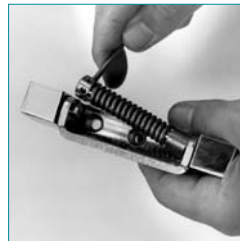
2. Slip bushing over hexagon pin on mounted hinge; then insert adjustment pin into adjustment bushing assembly.
