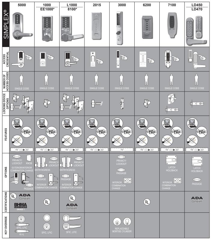
\* 8100 and EE1000 series fit 1 3/4" to 2 1/4" door thickness
