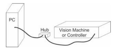
Once the machine is connected to a hub or router, and the hub or router is connected to your computer's network port, turn the machine on. The power switch for the Engrave-IT Pro is located below the LCD screen on the front of the machine. After the machine has initialized (Goto Home will be displayed after initializing), plug the supplied USB drive into an available USB port on your computer.
