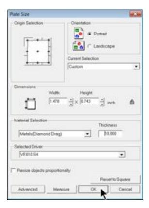
The machine will also allow you to outline the engraving area you just defined. Follow the instructions on your machine or controller to have the machine outline this engraving area with the red dot laser pointer. If the area appears to be correct. click on OK in the Plate Size window. The plate size in the Vision 9 software now shows the area defined with the measure feature. Design your job and send the job to the engraver.
