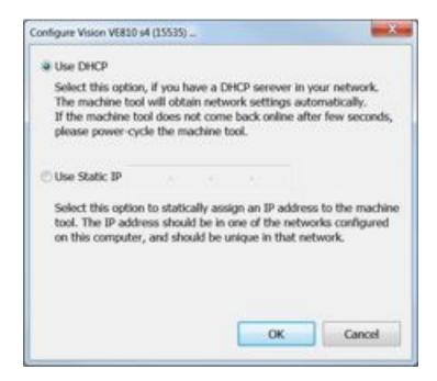
Set the IP address (as shown) to 192.168.5.101, then select OK. This sets the machine's IP address.
