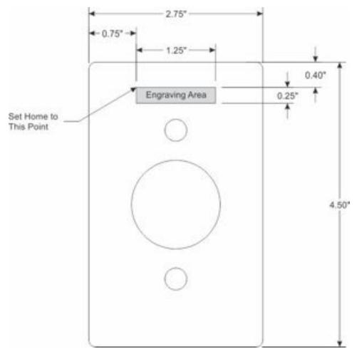
In this example, the user has identified the engraving area on an item, and the home (0,0) position of the machine will be set to match the upper left corner of the engraving area. Referencing the drawing above, the engraving area is 1.25 inches wide x 0.25 inches high.
