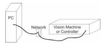
Once the machine is connected to your network with the supplied network cable, turn the machine on. The power switch for the Engrave-IT Pro is located below the LCD screen on the front of the machine. After the machine has initialized (Goto Home will be displayed after initializing), plug the supplied USB drive into an available USB port on your computer.
