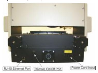
Connect the power cord to a 110 - 220 VAC source, then plug the power cable into the port on the back of the machine. Plug in the network cable (or the crossover cable) to the back of the machine and either plug the network cable into your network, your hub, or using the crossover cable, plug into the network port on the back of your computer.
