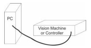
Once the machine is connected directly to your computer's network port with the crossover cable (the cable with green ends), turn the machine on. The power switch for the Engrave-IT Pro is located below the LCD screen on the front of the machine. Once the machine has initialized, the LCD screen on the machine will display Goto Home. Plug the supplied USB drive into an available USB port on your computer.
