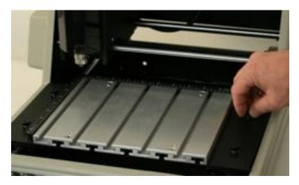
Remove the T-Slot table.
