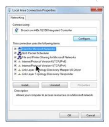
Select Properties, then select Use the following IP address: and enter 192.168.5.100 as shown. Then click in the Subnet Mask area, which will populate the correct location of 255.255.255.0. Select OK and close any other network configuration windows.
