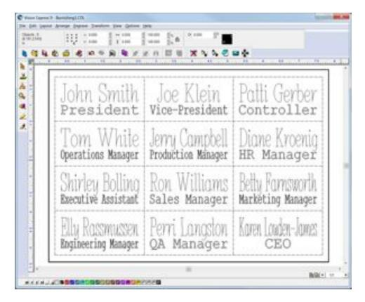
Also, if there are more variables than can be fit into one plate in the Vision software, multiple plates (or pages) are automatically generated for individual output to the engraver. The lower right corner of the Vision software screen allows the user to view the individual pages. During the Engrave operation, the user will select the page to be sent to the engraver.
