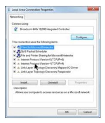
Then select Properties. Select Use the following IP address: and enter 192.168.5.100 and set the Subnet mask to 255.255.255.0 as shown. Then select OK and close any other network configuration windows.
