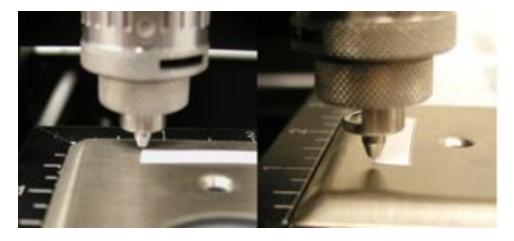
To set this point as the Home Position, press the Set Offset button on the engraver. A message will appear on the LCD Display reading "Home Set."
