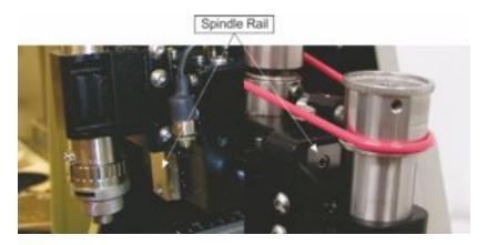
Move the Spindle down to expose the Z-Axis leadscrew for cleaning. Apply isopropyl alcohol to a paper towel and wipe down the Z-Axis leadscrew.
