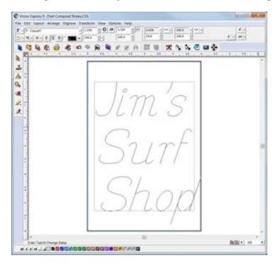
Once the file has been set up, select the Engrave Icon and click on the Tool Setup icon to open the Tool Setup Window, then from the Materials selection drop down list, select Engravers Plastic(Engraving) and click on OK. In the picture below, the Cut Toolbox shows that the Vacuum, Prox, Dry Run, and Spindle are all enabled. Since this is the second example job, sending a Dry Run job to the engraver is suggested. Select the Engrave Icon to send the file to the engraver.
