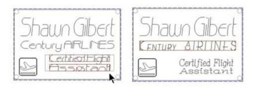
At this point, we need to change the two fixed text fields to graphics, so that when we import the text file for multiple badges, the correct text is replaced. Select the two text fields shown and from the toolbar, select Arrange — Text To Graphics. HINT - to select more than one object, click on the first object, hold down the Shift Key, then click on additional objects.
