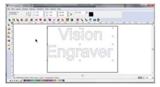
In order to align the text to the center of the plate, select Layout — Arrange and Distribute — Align to Sign Blank — Center (as shown below) from the top toolbar. Note that there are several ways to align objects within the Vision software.
