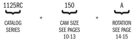
Example: 1125RC150A - 1 1/8", removable cam, spring clip mounting, 2" straight cam, 90° CW rotation, key removable in locked and unlocked positions.
