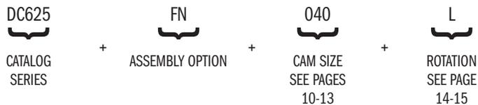
Example: DC625FN040L - 5/8" dust cover, fixed cam, nut mounting, 5/8" straight cam, 90° CW rotation, key removable in locked position only.
