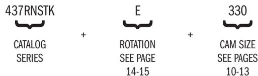
Example: 437RNSTKE330 - 7/16", stacked washer, nut mounting, 90° CW rotation, 1" hook cam bulk, key removable in locked position only.
