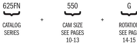
Example: 625FN550G - 5/8", fixed cam, nut mounting, 3/16" offset X 1 1/2" cam bent out, 90° CW rotation key removable in locked and unlocked positions. Also indicate keying, options, & accessories
