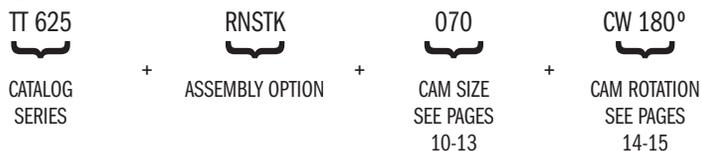
Example: TT625RNSTK070CW180° - 5/8, removable cam, nut mounting, 1" straight cam bulk, 180° CW rotation
