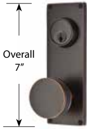
• Bern Knob with Keyed Modern Plate • Two standard 2 1/8" door preps • 3 3/8" Center to Center hole spacing
