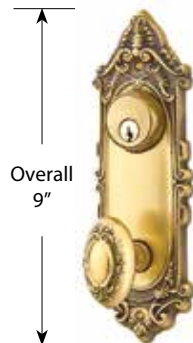
• Victoria Knob with Keyed Victoria Plate • Two standard 2 1/8" door preps • 3 5/8" Center to Center hole spacing
