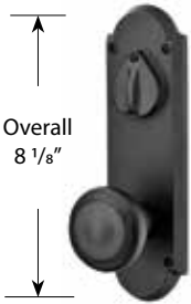
• Butte Knob with Keyed #5 Plate • Two standard 2 1/8" door preps • 3 5/8" Center to Center hole spacing
