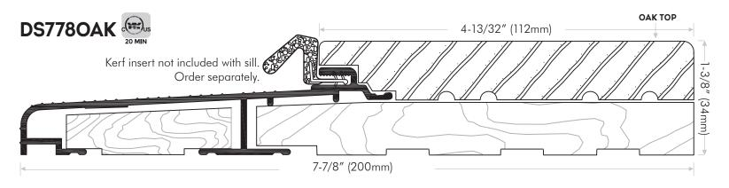
**DS778AOAK** Extruded aluminum sill, mill finish with interior oak top
