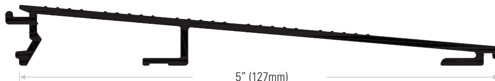
DS1115A150 Extruded aluminum mill finish. Length available: 150" (3810mm) only
