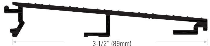
DS1135A150 Extruded aluminum mill finish. Length available: 150" (3810mm) only
