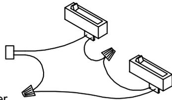
Installer must cut and reconnect orange wires from both breakaway switches to one Molex plug as shown
