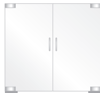
Paired Doors With Floor Closers
