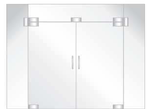
Paired Doors, Transom, and Sidelites With Floor Closers
