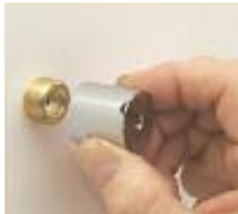
Place Base onto Threaded Insert and Fasten
