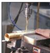
Drilling Holes in Tubing
