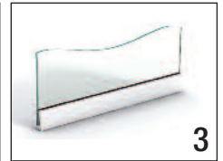
Roll in the Glazing Vinyl and You Are Done.
