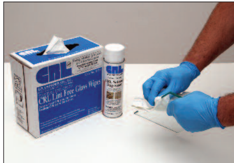
Second, clean the edges to be bonded with Cat. No. CRL7528 Cleaner and Degreaser
