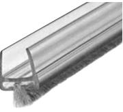
This CRL Clear Polycarbonate with Pile Weatherstrip prevents drafts from entering between glass doors. Simply snap over the edge of 1/2" (12 mm) glass. No tools required to install. Recommended clearance is 5/16" to 3/8" (8 to 10 mm). Stock lengths measure 98" (2.49 m) and can be shipped U.P.S.
