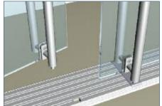
Glass Mount Detail at Latch With Threshold Prepped for Latch
