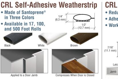
CRL Self-Adhesive Weatherstrip is designed to be applied to the "stop" perimeter of a frame to prevent energy loss, reduce noise and dust infiltration. It will not crack or craze in cold or heat. Self-adhesive application makes installation easy and requires only scissors or a utility knife to cut to size. Tested in accordance with ASTM E-283 and listed by Warnock Hersey for use on labeled openings up to 90 minutes.
