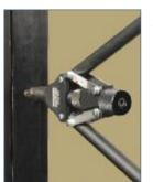
Third, compress the Rivet-Nut by using the CRL Cat. No. 34604 Heavy-Duty Thread Insert Tool
