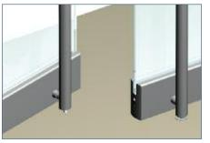
Rail Mount Detail at Latch at Floor With AMR209PS Dustproof Keeper
