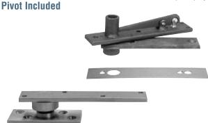
This Rixson<sup>®</sup> Center-Hung Pivot Set features a 500 pound (227 kg) weight capacity, and can be used on doors up to 44" x 102" (1118 x 2591 mm). Double-acting non-handed Bottom Pivot mounts directly to floor. Sealed bearings for protection against the weather.
