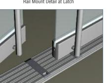
Rail Mount Detail at Latch With Threshold Ramp Strike
