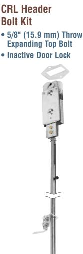
Our DL2240 Series Header Bolt is designed to add a top-door locking point in the inactive door. This bolt is activated when the DL2110B or MS18533 Latch is locked. As the throw bolt locks into the inactive door, it lifts the adjustable nylon rod end causing the Header Bolt to lift and expand its pawls in the head, which centers the bolt into the header. One per package.
