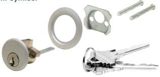
This Rim Key Cylinder comes with two keys in the Schlage "C" keyway configuration. 1-7/8" (47.6 mm) break-away screws and 1-1/4" (31.8 mm) break-away spindle standard. They are available keyed different or keyed alike in satin aluminum or dark bronze finishes. One per package.
