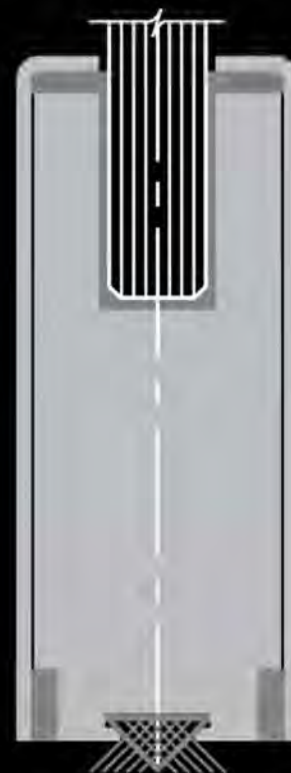
BRONZE OR STAINLESS STEEL FULL SIZE SECTION THRU BOTTOM AND TOP RAIL
