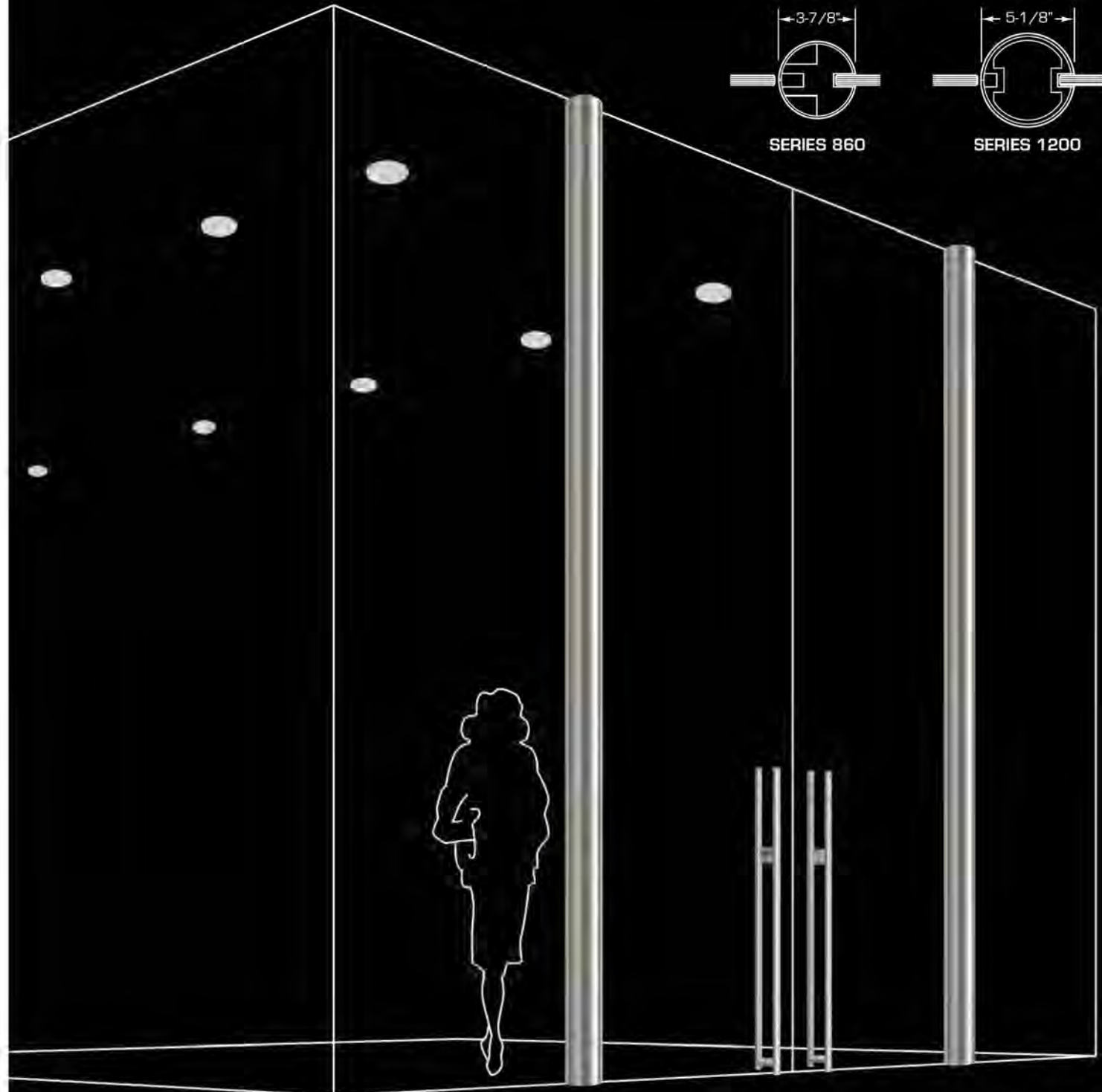
SERIES 1200 DOORS WITH DB-140-KS DEADBOLT HOUSINGS
