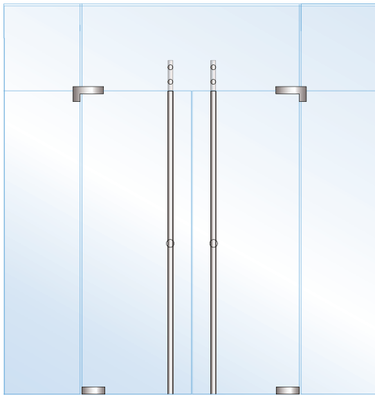
Double Door Installations Require Two Locking Handles
