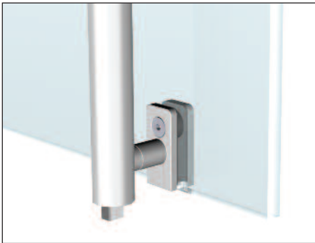
Glass Mount Detail at Latch
