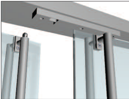
Glass Mount Detail at Latch With Header and PK Strike
