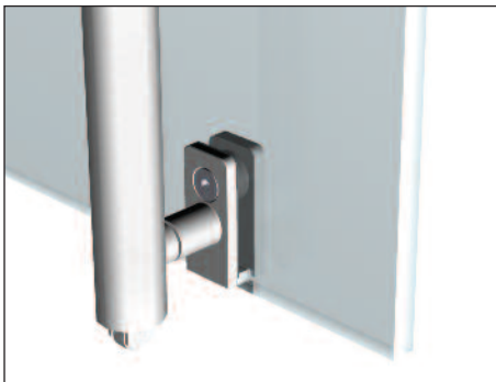
Glass Mount Detail at Latch
