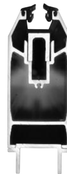
Reversible Saddle Positioned for 3/4" (19 mm) Clearance
