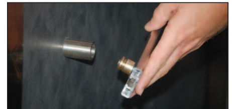
Secure Slide Fittings to Mounting Studs with Set Screws
