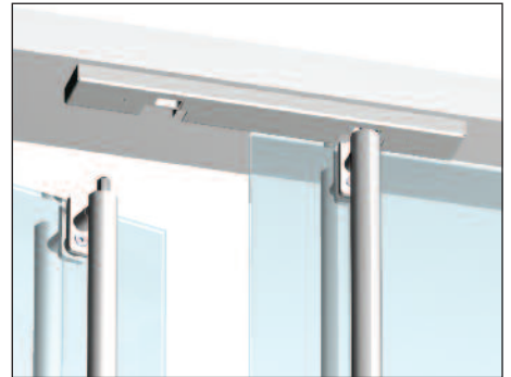
Glass Mount Detail at Latch With Header and ESK Strike
