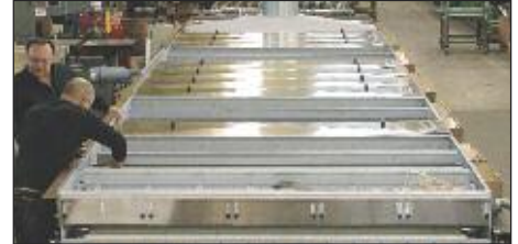
CRL Mirror Line Oven Sections are installed in the production line for testing before delivery.
