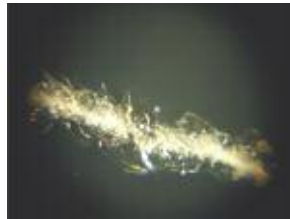
HEAVY/DEEP SCRATCH – Above is a magnified image of a heavy/deep scratch. It cannot be removed with this system.
