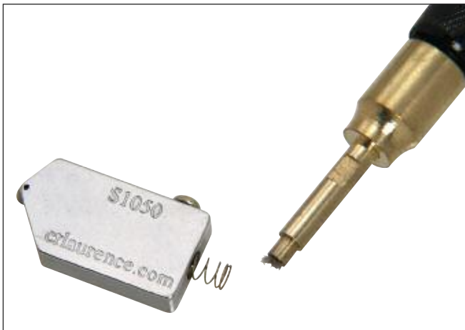
Spring-Loaded Cutting Head and wick extending into the handle oil reservoir to provide continuous lubrication
