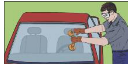
Set the Auto Glass Setting Stick™ out of the way and you are now ready to place the glass in position.
