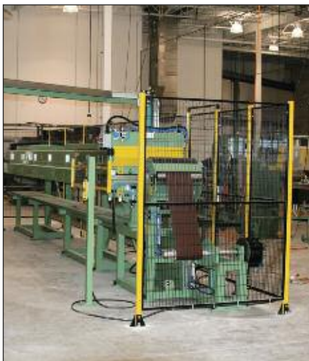
The Roll Slitting Machine accommodates a 55' wide x 600' long (1397 mm wide x 182 m long) roll of belt material and performs multiple precision cuts into 12" (305 mm) wide lengths.
