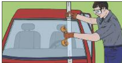
After setting your side, walk to the other side, lift the stick up a small amount and slide the Auto Glass Setting Stick™ out of the way.
