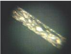
LIGHT SURFACE or SCUFF MARK SCRATCH – Over 95% of all scratches are light scratches or scuff marks. This magnified image above shows a light scratch. This scratch can be removed.
