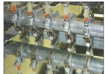
Cutting Heads on a CRL/Somaca Stalter Machine in action, cutting mirror strips.
