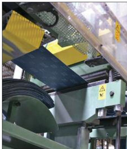
The Cut-to-Length Machine then cuts the abrasive cloth material into various overall lengths to make abrasive belts.
