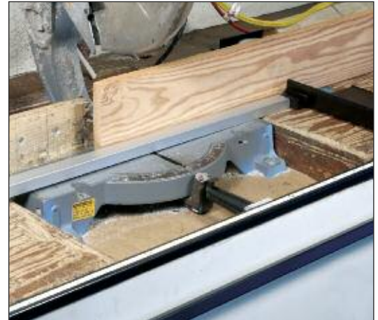
Snow Cut-Off Gauge in Installed Position
