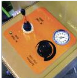
Pneumatic Pressure Controls and Joy Stick for Drill Motors
