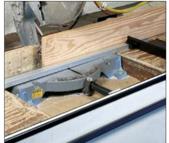
Snow Cut-Off Gauge in Installed Position
