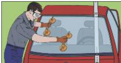
Set the glass on the peg at the bottom of the Auto Glass Setting Stick™. It is held in place while you put your side where you want it.
