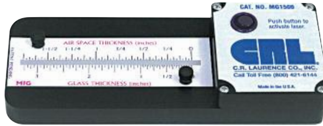
Overall Insulating Glass Thickness Scales
