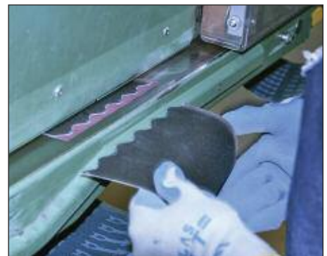
The 1-1/8", 3" or 4" (3, 76, 102 mm) wide belts are then fed into the Scuffer/Gluer Machine which:
