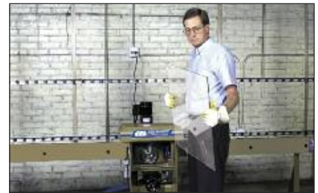
Fill Coolant Tank and start edging glass
