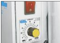
Electronic Variable Speed Control
