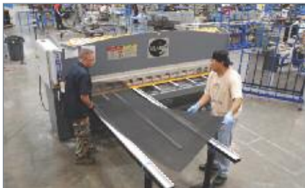
Shearing High Tensile Mesh in Our Los Angeles Manufacturing Plant
