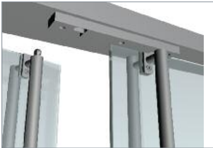
Glass Mount Detail at Latch With Header and PK Strike
