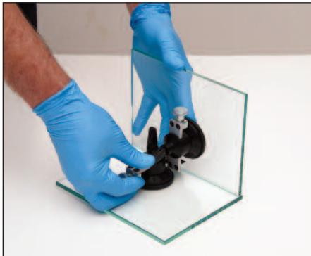
2. Apply Fixtures and Align Joints
