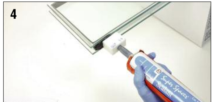
4 Apply CRL Hot Melt Butyl or Cat. No. 877 Super Spacer Sealant to seal the unit
