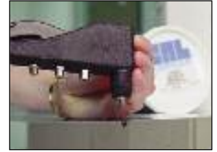
4. At maximum pull, the mandrel breaks (at the pre-cripped section) and is withdrawn. The mandrel head remains locked in the rivet, closing the rivet bore.
