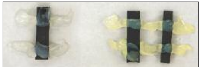
TPR Blocks will not discolor applied sealants like neoprene blocks can.
