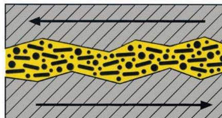
SILARAMIC prevents metal-to-metal contact under conditions of high loads and dampens noise.
