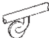
-25 Underslung Welded Support
