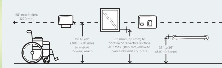
Dimensions change if mounted over counter or lavatory. Operable parts must be beneath maximum height.
