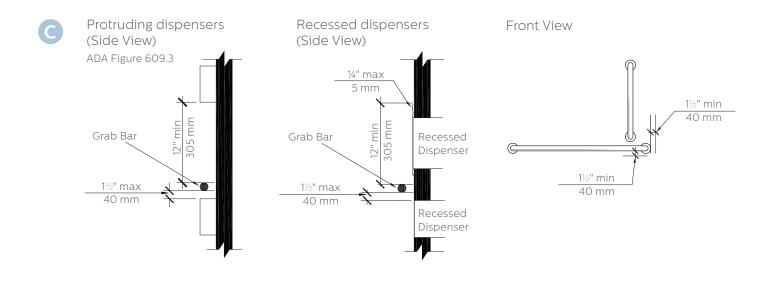
Dimensions for rear grab bar installation. Rear wall grab bars shall be 36" (915 mm) long, and mounted so 24" (610 mm) are to the transfer side of the toilet and the other 12" (305 mm) to the wall side. The rear grab bar can be split or shifted to the open side to accommodate the required location of the flush control valves.
