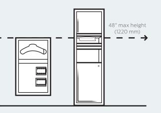
In order to create a safe environment for visually impaired patrons, fixtures must be detectable with a cane. The diagram above highlights this requirement.
