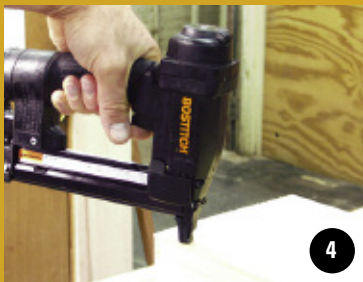
Caseback being secured with 18-gauge SL staples
