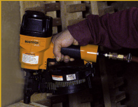
N58C Coil nailer fastening fence header board
