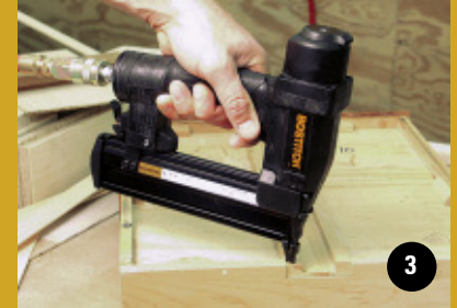
18-gauge brads fastening quarter round
