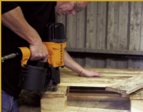
N400C-1 Nailing mat to block pallet
