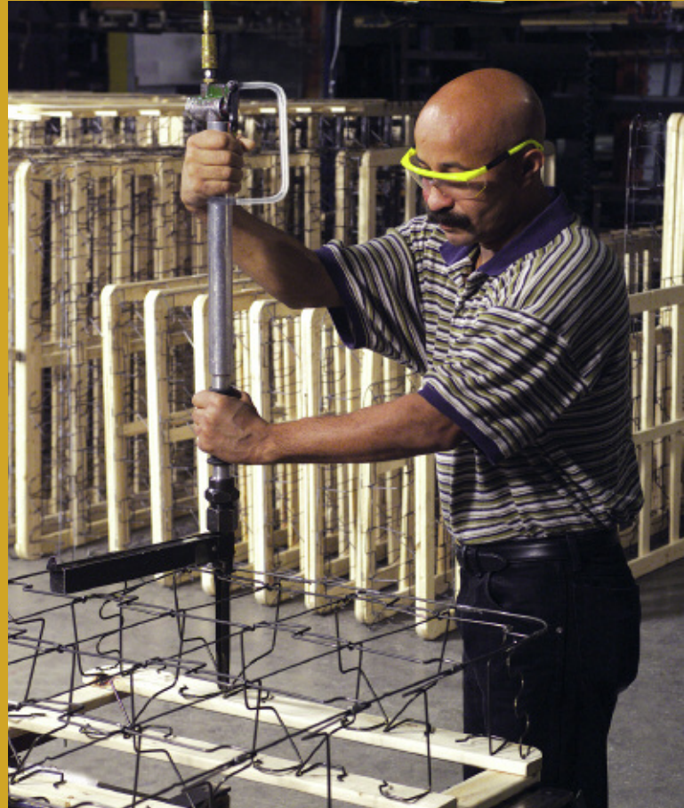
BCAR-2S Stapler foundation spring to flat
