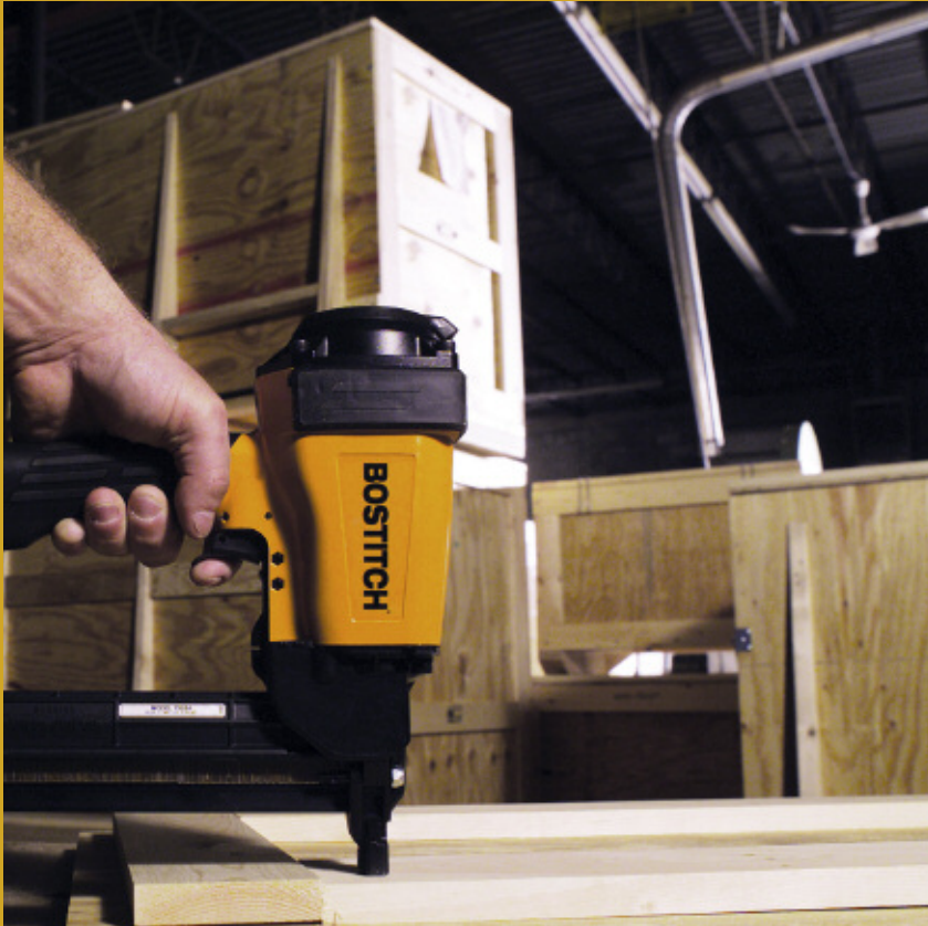
750S4 Assembling crate face-frame
