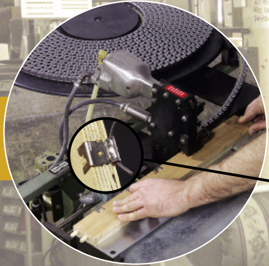
Sinuous spring anchor clip application to chair rail w/ AK Machine
