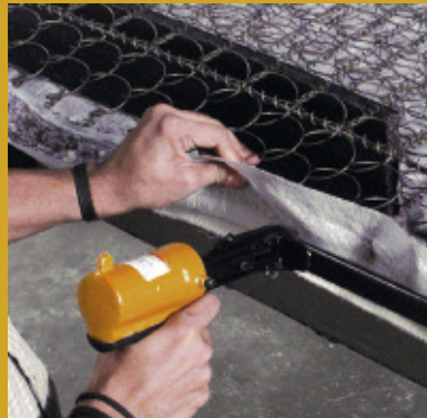
TR203 D-Ring tool connecting flange to innerspring
