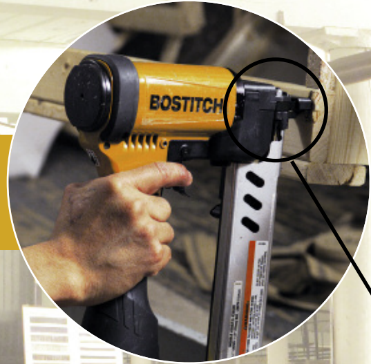
538S4 Stapler applying staples during knock-up
