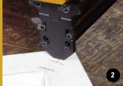
CF15 Applying corrugated fastener to an angled butt joint
