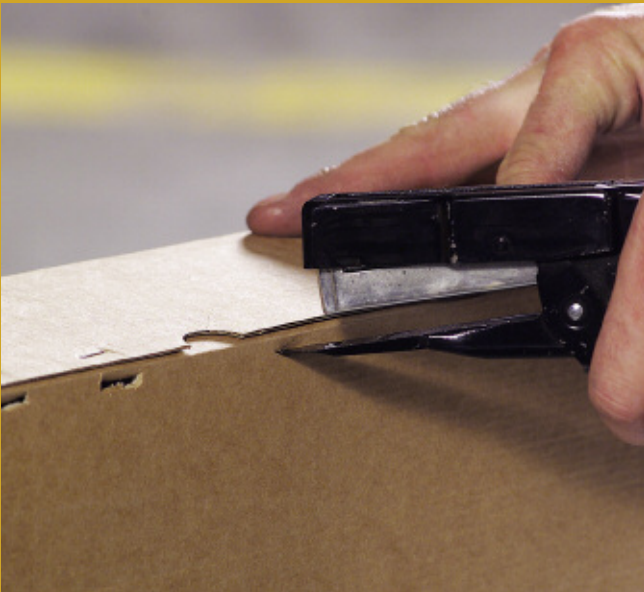
P6C-8P With pointed anvil piercing corrugated to seal container from outside
