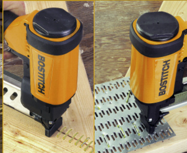
538S214-1 With 14-gauge staples stitching truss joint and truss plate prior to roller press
