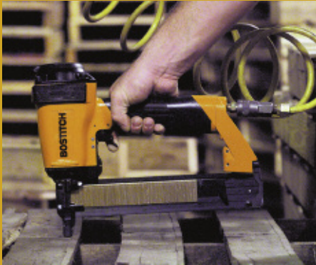
750S4 Reattaching Deck Board
