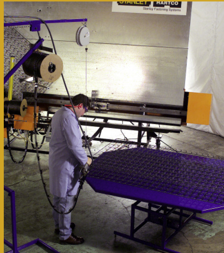
Coil clip system and vertical rotating clip machine securing innersprings to borderwire
