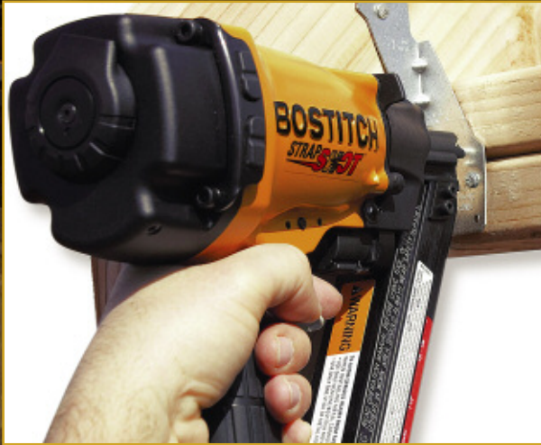
MCN150 Fastening Hurricane Strap to framing joists
