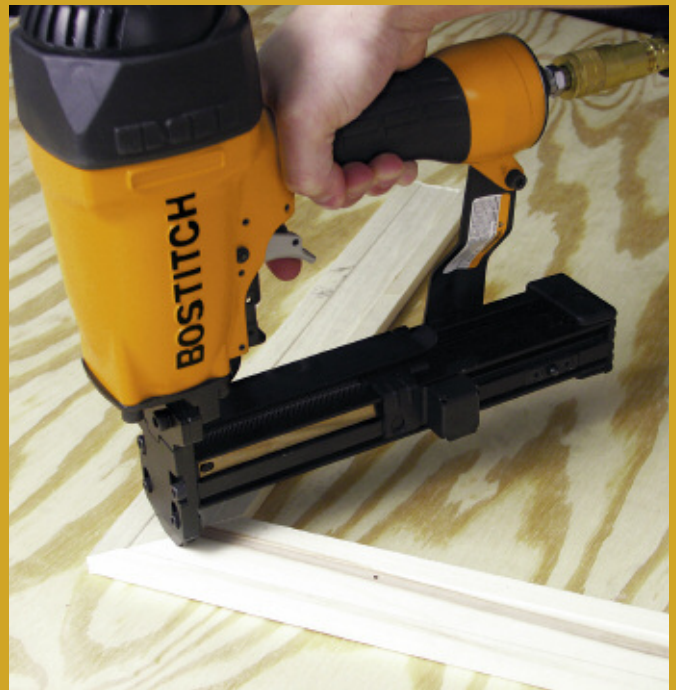
CF15 Corrugated tool applying mitre fastener to window frame
