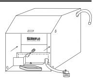
2. Screw Soap Supply Line Cap to Cartridge Outlet by turning clockwise. Soap should flow through the tubing.
