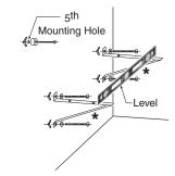
5. Route tubing through hole in cabinet side panel or back wall.
