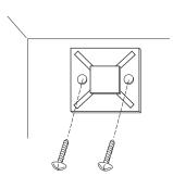
11. Attach intermediate tubing to cable supports with the cable ties between soap pumps
