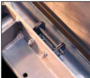
Concealed Stainless Steel Hinges
