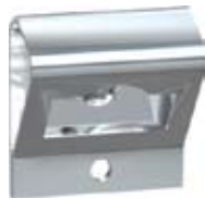
0711-B BOTTLE OPENER One piece, 16 gauge type 304 stainless steel with bright finish. Projects 1 1 / 16 " (27 mm) from wall, 2" (50 mm) wide x 2 1 / 4 " (55 mm) high.
