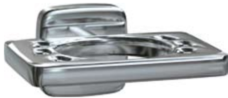
7335 TOOTHBRUSH AND TUMBLER HOLDER Similar to 7320 Soap Dish. Has 2¼" (60 mm) diameter hole in center of unit to hold tumbler. Accommodates 6 toothbrushes. 4¼" x 2" (110 x 50 mm); projects 4" (100 mm) from wall.
