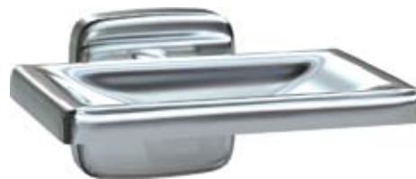
7320 SOAP DISH Drawn, one-piece soap dish welded to support arm and flange. Has two drain holes and two ridges to support bar of soap. 4¼" (110 mm) wide, 2" (50 mm) high; projects 4" (100 mm) from wall.
