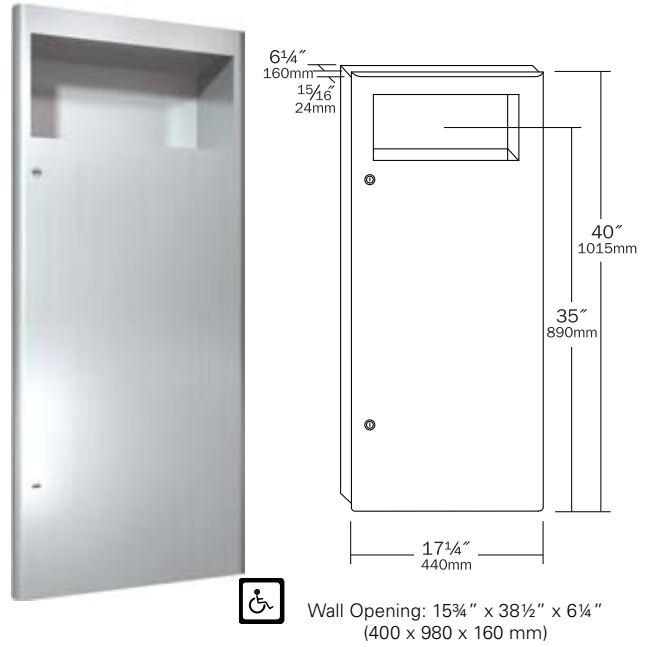
9474 WASTE RECEPTACLE Waste receptacle is 12 gal. (45.4 L) stainless steel.
