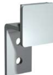
8425 CLOTHES HOOK Heavy duty 11 gauge type 304 stainless steel with satin finish. Hook projects 1¼" (32 mm) from wall and is 2¼" (55 mm) high.
