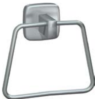
7385 TOWEL RING For bath and hand towels. Ring is 4½" (115 mm) wide, made of ¼" (6 mm) diameter stainless steel bar. Projects 2½" (65 mm) from wall. 5" (125 mm) high.
