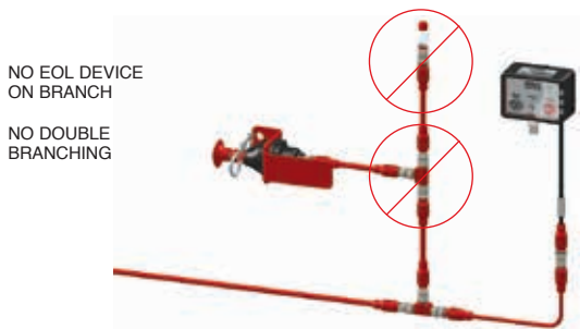
FIGURE 5-34 INCORRECT EMA INSTALLATION 009197
