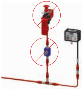
FIGURE 4-9 INCORRECT EMA INSTALLATION 009199
