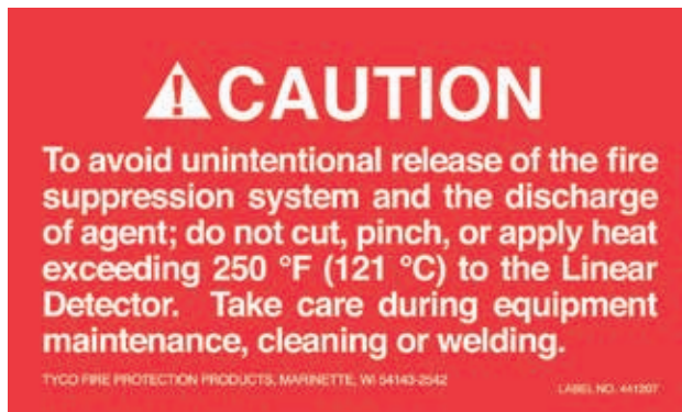
FIGURE 2-28 LABEL FOR PROTECTING LINEAR DETECTOR 009325
