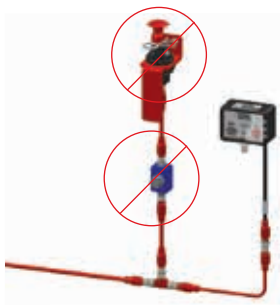
FIGURE 4-10 INCORRECT EMA INSTALLATION 009200
