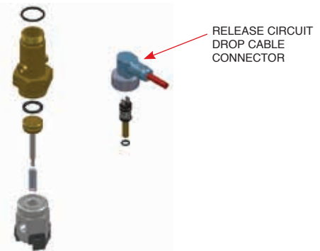
FIGURE 8-9 ELECTRIC-PNEUMATIC ACTUATOR RETAIN ALL PARTS FOR RE-ASSEMBLY 009244
