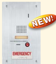
IS-SS-RA-R ADA Compliant Audio Only Door Station with lettering and Braille signage, LED call status indicator, single call button, 2 form C relay outputs, stainless steel, flush mount
