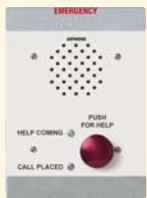
NE-NVP-RA Door Station, powder- coated steel, red mushroom call button, call status indicators, braille signage, flush mount, 3-gang
