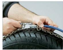
Reach around with both hands and grasp the ends of the coated side cable. Pull both ends to the top of the tire and fasten the inside hook. Be careful to avoid twists in any part of the chain.
