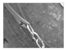
Connect the outside fastener at it's loosest setting, then pull the cable towards you to create as much slack as possible. Make sure that none of the cross members are caught in the "shoulder" area of the tire tread.
