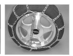
SCC recommends chain tighteners (sometimes known as chain spreaders) be used to take up additional slack. To make this simpilar, attach the first hook at the "11 o'clock position", next at the "5 o'clock position" and so forth. The open side of the hooks must face away from the tire. No further adjustment is necessary.
