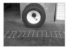
Park vehicle on firm level ground, away from traffic. Unroll the set and lay each half pair on the ground next to the tire it is intended to cover. Make sure that there are no twists or kinks in the cable chain.
