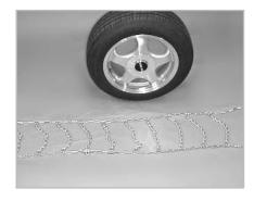
Park vehicle on firm level ground and turn off the engine. Set the parking brake. Unroll the chains and lay them out flat making sure there are no twists or tangles. Make sure the smooth side of the cross chain hooks are toward the tire.
