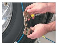
Roll 1/4 of a tire revolution onto the chain. Connect the inside speed hook.
