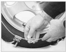
Take the bushing end of the lower fastener and thread it through the keyhole (the one near the ground) using the same process as the top fastener. Please see below for a detailed look at making this connection.
