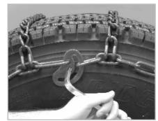
Cam side chain adjusters should be closed by turning the cam clockwise with the included cam tightening tool. If there are more than 2 "loose" links at any of the fasteners, we recommend that you secure them to the side chain with a piece of wire or a plastic tie.
