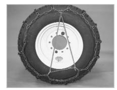
SCC recommends chain tighteners (sometimes known as chain spreaders) be used to take up additional slack. To make this simpler, attach the first hook at the "11 o'clock" position, the next at the "5 o'clock" postion and so forth. The open side of the hooks must face away from the tire. No further adjustment should be necessary.
