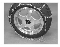
Pull one cross chain down to the point where the tire meets the ground. Move the vehicle so that 1 or 2 cross chains pass under the tire.
