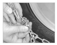
Reach behind the tire and fasten the inside connector on the 2nd or 3rd link.
