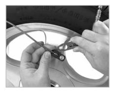
Grasp the outside cable with both hands and pull it toward you to create as much slack as possible. Connect the top fastener.
