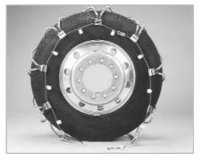
Park vehicle on firm level ground, away from traffic and turn off the engine. Set the emergency brake. Drape chain over the tire. Make sure that the smooth side of the crossmember hooks is against the tire sidewall. The tightener hooks on the side cable must be on the outside of the tire (towards you).
