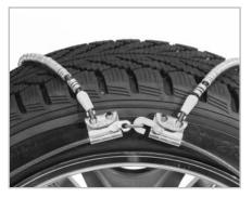
Reach around each side of the tire and grasp both ends of the non-split cable (the cable that is furthest away from you). Pull both ends to the top of the tire so the fasteners can be seen and manipulated more easily. Connect the inside fastener.
