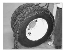
Park vehicle on firm level ground, and turn off the engine. Set the parking brake. Lay the tire chains out flat on the ground, making sure there are no twists or tangles. Make sure the cross chain hooks are facing upward.
