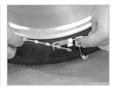
At the inner sidewall, make the connection on the inside of the tire by pushing the cable with the end bushings behind the tire and toward the front of the vehicle.
