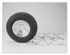
Park vehicle on firm level ground, away from traffic and turn off the engine. Set the emergency brake. Remove any wheel covers. Chains should be installed on drive tires. Lay the cable chain on the ground with the smooth side (TIRE SIDE) of the cross member hooks up.
