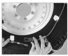
Take the bushing end of the lower fastener and thread it through the keyhole (the one near the ground) using the same process as the top fastener. Please see below for a detailed loot at making this connection.
