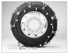
Roll onto the chain by moving the vehicle forward two or three feet (60-100 cm). Which is the equivalent to 1/4 of a tire revolution.
