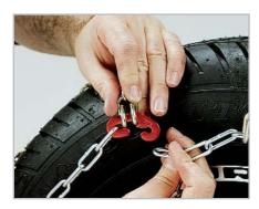
Hook the red end fastener on the outside side chain to a corresponding link of the side chain at the top of the tire. Then hook the silver end fastener to the side chain at the bottom of the tire.
