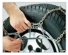
Attach the rubber tensioner to equal segments of the side chain, as shown. Make the first connection at about the "5 o'clock position", the second at "11 o'clock" and so on. Hook any excess side chain with a rubber tensioner hook or wire tie.
