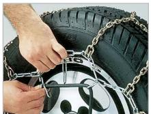
Disengage the rubber tightener and unhook the outside side chain, then the inside hook fastener. Reach behind the tire and pull the hoop apart and off of the tire, so that it is laying flat on the ground. Then drive off the chain.
