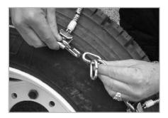
Connect the "speed hook" on the inside of the tire (the side away from you). As a starting point, we recommend that you fasten it so that there are no more than two "free" links. It may be necessary to drive forward two to three feet so that the inside connection can be made more easily.
