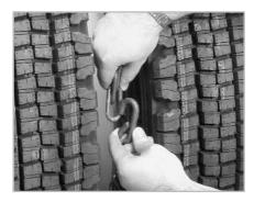
Reach behind the tire and engage the inside connector making sure it is as tight as possible. Then connect the center (between the duals) fastener in the same manner. See the illustration below for a detailed look at this connection.
