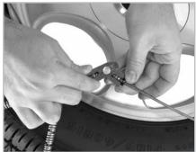
Connect the bottom fastener. In order to close the outside fasteners, the opposing ends must be at an angle of approximately 30° to each other.
