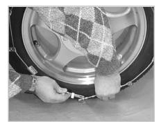
On the outside of the tire, thread the cable with bushings through the end hook for initial mounting. Grasp the outside side cable with both hands and pull it towards you. This will create as much slacks possible. Then make the outside connection in the same manner.
