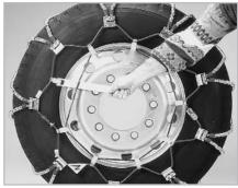
Install the rubber tensioner, always stretching the tensioner from one hook to the one farthest from it (use the included lever tool to make this installation easier.)
