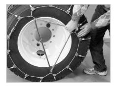
Install the rubber tightener. Always stretching the tightener from one hook to the next farthest from it. Make sure that the tightener hooks are facing away from the tire. If hooks are not facing away from the tire, damage will occur. Chain may now be driven without further adjustment.
