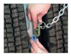
Reach behind the tire and fasten the inside connector making sure it is as tight as possible.
