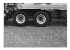
Park vehicle on firm level ground, away from traffic. Unroll the set and lay each half pair on the ground next to the tires it is intended to cover. Make sure that there are no twists or kinks in the cable chain. Make sure that the smooth side of the eyelets (marked "TIRE SIDE") will be against the tire. If the smooth side will not be toward the tire, damage will occur
