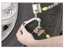
Connect the outside latch fastener and secure with floating link. (Actual lever is black, but pictured here as silver for easier identification.
