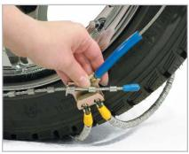
Repeat this process with the gold adjustment fastener. Ensure that both fasteners are adjusted within one bead of each other. Move the vehicle a few feet. Remove cable "slack" by retightening both adjustment points as equally as possible.
