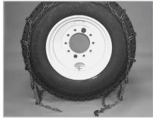
Make sure the cross chain hooks are facing upward. Hooks that face down (towards the tire) will cause damage to the tire.
