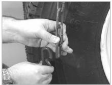
Next fasten the outside fastener in the same manner, again making sure it is as tight as possible. Drive a short distance and retighten all fasteners. For best results, make sure fasteners are adjusted equally and as tight as possible.
