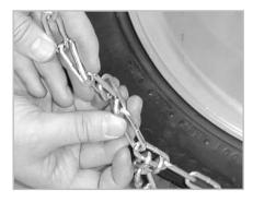
Reach behind the tire and engage the inside connector on the 2nd or 3rd link. See the illustration below for a detailed look at making this connection.
