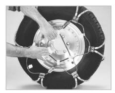
Attach the rubber tensioner to take up the additional slack. To make this simpler, attach the first hook at the "6 o'clock" position, the next at the "12 o'clock" position and so forth. The open side of the hooks must face away from the tire. No further adjustment is necessary.
