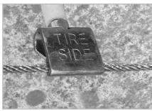
Make sure that the smooth side of the eyelets (marked "TIRE SIDE") are against the tire. If the smooth side is not toward the tire, damage will occur.
