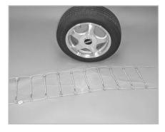
Park vehicle on firm level ground, away from traffic and turn off the engine. Set the emergency brake. Chains should be installed on drive tires. Unroll the chain on the ground next to the tire. Position the cable so the end hooks are toward the front of the vehicle.
