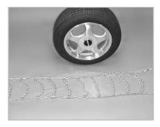
Park vehicle on firm level ground and turn off the engine. Set the parking brake. Unroll the chains and lay them out flat on the ground, making sure there are no twists or tangles. Make sure the cross chain hooks are facing upward.
