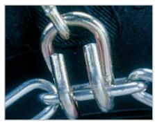
The curved portion of the cross chain hooks should face away from the tire.
