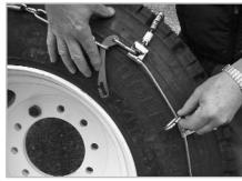
Fasten the outside connector by passing the long lever through one of the chain links, folding it back in the opposite direction and securing the "keeper" link on the end of the lever. If care is taken to make this connection as tight as possible, it may not be necessary to retighten after driving. If you find that the inside fastener also has to be adjusted to assure a snug fit, you should do it before fastening the outer fastener.
