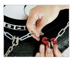
Drive vehicle off highway to safe level ground. Turn off the engine and set emergency brake. The wheel should be positioned so that the red plastic marker is <u>not</u> at the 12 o'clock position on the tire.
