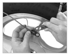
Grasp the outside cable with both hands and pull it toward you to create as much slack as possible. Connect the top fastener.
