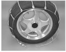
Drape the chain over the tire so that the smooth side of the cross member hook is against the tire. The cross member nearest the end hook should touch the ground.
