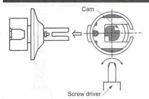
(1) Locking Turn key counter-clockwise. Return to take a key out. (2) Unlocking: Turn key clockwise. Return to take a key out.
