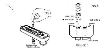
b) Can also be changed to 6-digits by adding the identified wafers and to 4-digits by adding the neutral wafers (one pc each of spare identified and neutral wafers attached)
