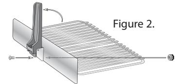
Step 6: Using attaching hardware found in the parts bag, take one large bolt PN# LS-501 and one large thumb nut PN# LTN-501. Slide large bolt through the round hole, capturing the loop, handle bracket and the food rack cover. Thread the nut onto the large bolt from the opposite of the food rack and tighten (Figure 3).
