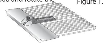
Step 5: Rotate handle and food rack cover towards you together as a single unit (Figure 2).
